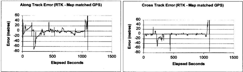
Figure 6. Cross-track and along-track errors for map-matched GPS.
