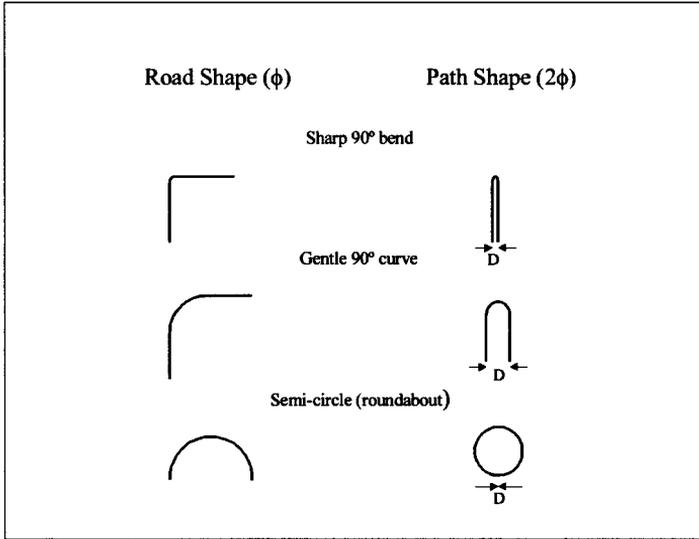
Figure 3. Basic road shapes can be transformed into path shapes with twice the curvature, which can then be interpreted in terms of favourable geometry (MDOP).
